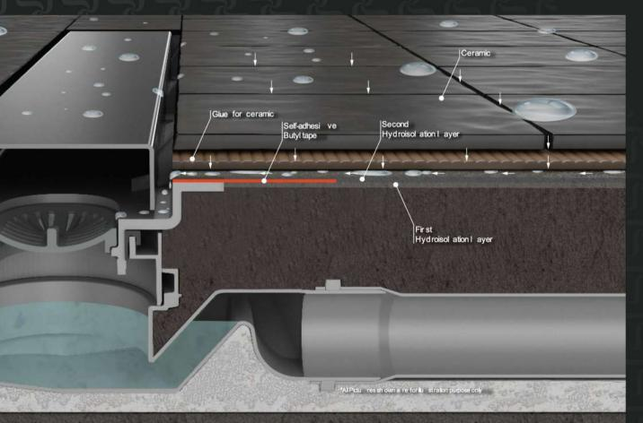
During the years, water in bath room has tendency to build under the tiles as consequence of erosion of grout and moisture in the bath room. Usually it takes 5-7 years until this problem happens and then a leakage shows up in a place
